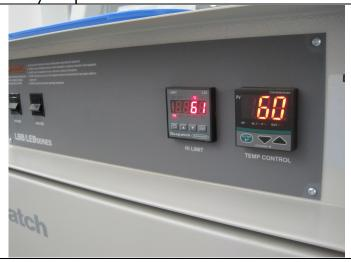
2. Turn on the heater for the ultrasonic cleaner chamber. The switch is on the back of the chamber. The chamber temperature should be set at 50-60C.
