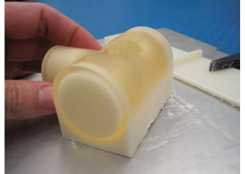
6. Place the part in the oven. Ensure that the wax-catching tray is in place below your part. The part will sit in the oven for awhile (~10-60 mins, depending on part geometry).
