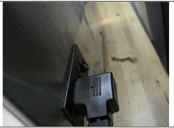
3. Remove the aluminum platform from the ProJet machine. Slide the small lever to the right and allow the latch to swing open.
