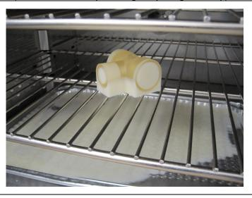
7. As the wax liquefies, you can move the part around to allow the liquid wax to drip off/out of your part.
