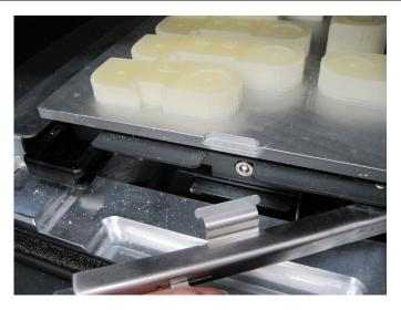
4. Lay the aluminum platform on a stable table. Gat a chisel and wooden mallet.
