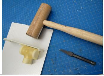
5. Place the chisel at a LOW angle against the base of each part. Tap the chisel GENTLY with the mallet. Some parts may need to be tapped in several locations. Be especially careful with thin and delicate parts.
